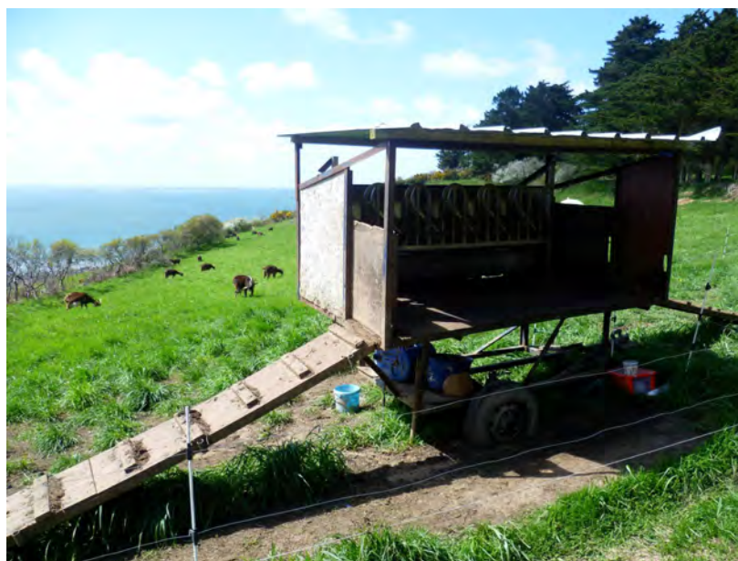
Figure 30. Dairy goats system using a wide range of rangelands in more humid northern France. Goats stay outside all year long. In winter, goats browse also nearby semi-evergreen shrublands. The mobile milking machine allows keeping the livestock also on remote pastures or rangeland (Photo A. Letort).
